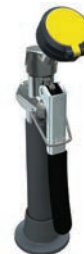
Hand Held Face Body Wash squeeze valve nozzle on 8' coiled hose and bracket. Can be used to rinse body parts while victim is sitting or lying down. Wall or hood mounted, 3/8 NPT, Barrier free. Cat No. 16005
