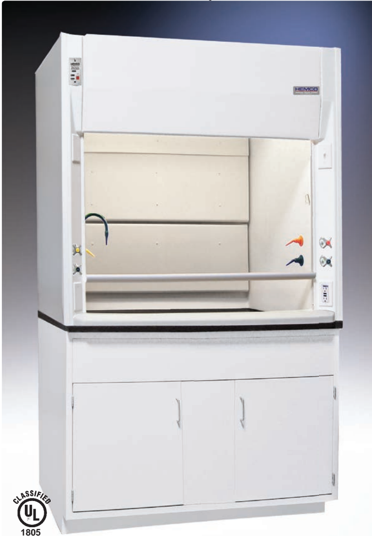
UniFlow LE Fume Hood Cat. No. 35521 shown with optional epoxy resin worksurface, base cabinet and fixtures See pages 20-25 for accessories.
