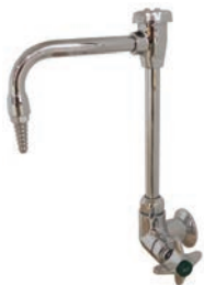
Water Faucet with Vacuum Breaker Cold water remote controlled 6" swivel gooseneck. Epoxy coated brass. Cat. No. 50023
